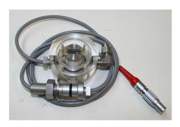
**S-wave transmitter** (P-wave receiver) Red LEMO plug
