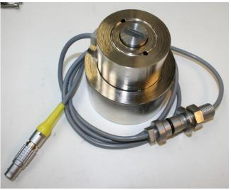
P-wave transmitter (S-wave receiver)
